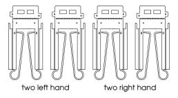
Drill #78 holes in the two grab iron holes and install grab irons of your choice (not included in the kit). These will help hold the assembly in place.
