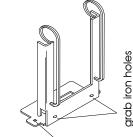
note offset stirrup step hole. this hole accepts 'plate' of stirrup step.
