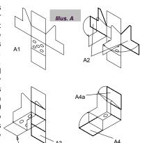
Once all of the locator boxes are bent to shape, liquid cement or contact cement them to the top surface of the deck where the old boxes were. Be careful not to cover the holes drilled for the
