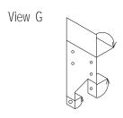
the side and two on the bottom for the stirrup steps. Drill holes using template instead of marking with pin as the precision is needed for placement of pins on the ladders.
