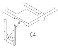
pins to the bottom side of the car so the flat side of the upright is flush against the side of draft gear. Using supplied .020" X .100" styrene, Using cut to .300" in length and liquid cement to bottom of draft gear covering upright pins sandwiching them in place.
