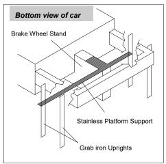
CA to the bottom of the brake wheel stand. Turn car right side up, and CA 'wings' to uprights so they are level. Cut .020 X .030 styrene to the same length of each wing and cement to top of each wing of the support. Touch up paint. Insert Step Up Platforms (#2) in drilled holes on end of car and cement to top of new support when platforms are level. Repeat on other end and touch up paint.
