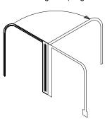
handrail bent shape). Keep in mind there is a left and right to these parts when bending. Insert the mounting pin οf these handrails in the holes of the supports #1 or #2. The longer
