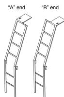
right to these parts. use diagram to the left for additional reference. Next bend the top half of the ladder back about 10 degrees just above the little hooks on each side of the ladder. Now bend the little hooks back 90 degrees in the same direction as the top of the ladder.
