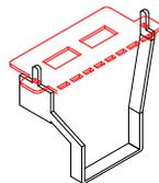
'left hand' Stirrup step formed to shape, shown inserted into holes on bottom of stanchion tab
