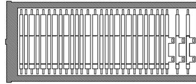
Shape of supports after trimming from fret - note fold lines dividing supports
