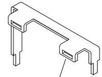
Shape of support #3 - note ladder loops bent down
