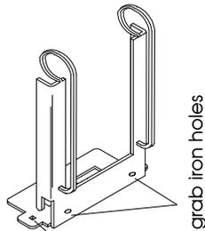
note offset stirrup step hole. this hole accepts 'plate' of stirrup step.
