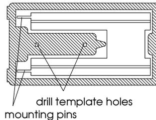
The brake housing stand should be mounted centered to the left of the coupler box. There are two drill template holes on the fret holding this piece. Position and drill holes where you are comfortable with. Bend sides of brake housing stand over 90 degrees and install in drilled holes. Brake housing and hardware is your choice.
